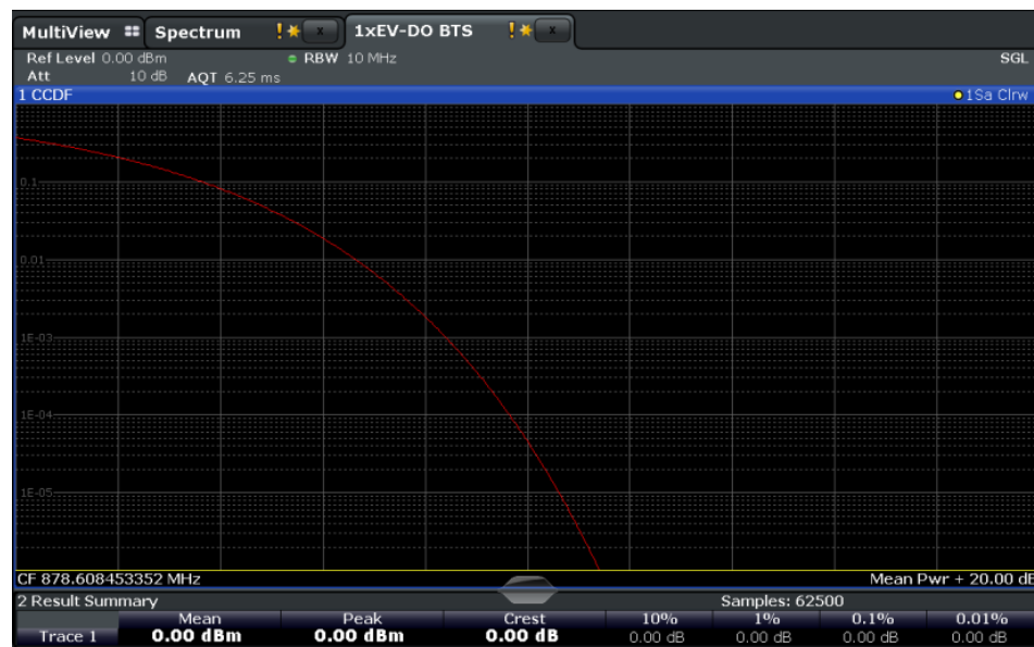
Fig. 3-26: CCDF measurement results in the 1xEV-DO BTS application
