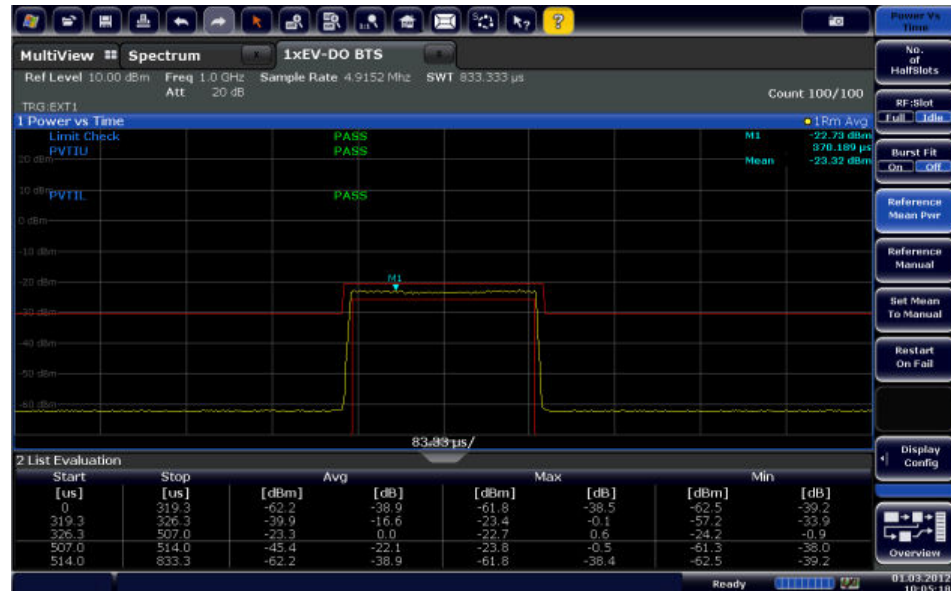
Fig. 3-21: Power vs Time measurement results in the 1xEV-DO BTS application
